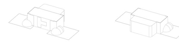
Note: The amount of solder paste applied as shown in the picture is just for illustration purpose only. When mounting and soldering the LEDs, avoid excess solder paste from overflowing onto or near the epoxy lens.
